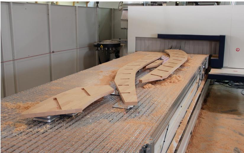
producing several posts simultaneously. Only when the machine has finished all steps with one tool on all posts, the tool is changed and the machine proceeds to the next step with the new tool. The processing of 4 posts now takes about the same amount of time than 2 posts required before Luxholm made the change.
