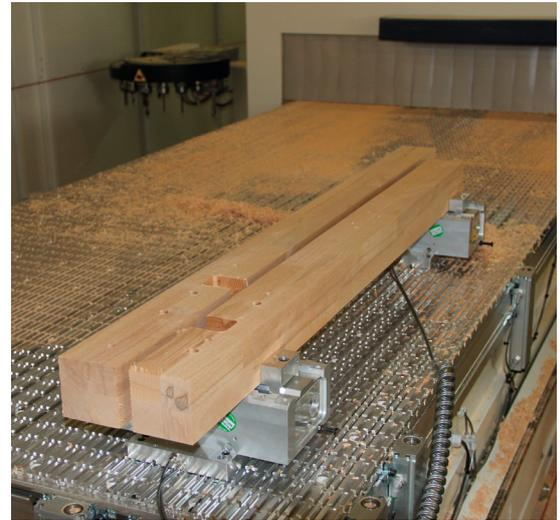
Since the processing of posts generally requires many tool changes, the stair builder saves even more time by utilizing tool optimization and producing several posts simultaneously.
