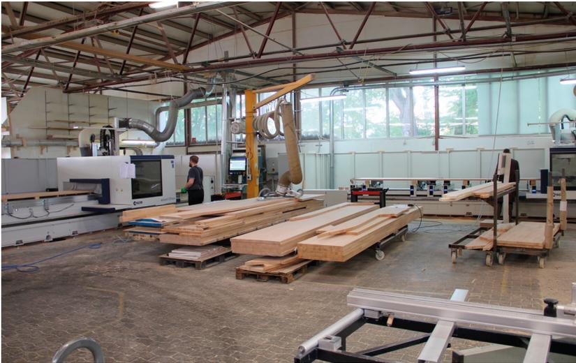
During a normal work day, one of the Accord 25 FXs is utilized for the processing of individual parts. The other machine, which is equipped with automated vacuum cups, has been configured for plate optimization and table arrangement.
