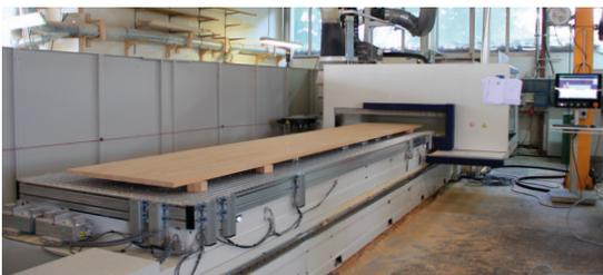
The maximum capacity on the machine is 8 stringers at a time. A possibility that promises future potential timesaving.
