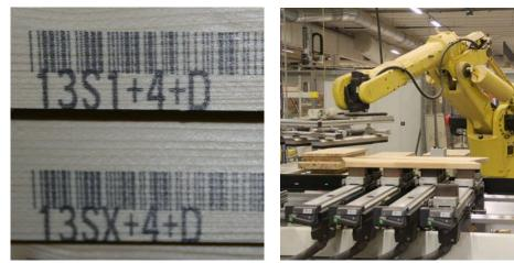
It is possible to use external data from other systems (ERP), which already include barcodes. The data is read in, clearly assigned to the respective CS-barcode (mapping), and can be used smoothly.
