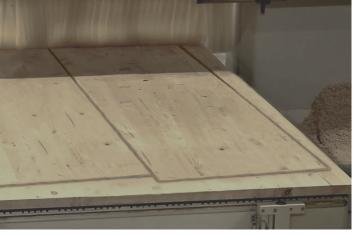
The optimization is possible to go with the grain or turned at a 90° angle.
