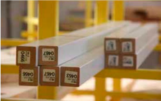
RFID chips on stair components enable complete traceability and full transparency in production.
