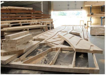
The stair builder is able to optimise small parts on the machine, which would not be possible on a specialised nesting machine because the vacuum cups would not be able to hold such small parts.
