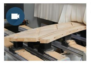
Another major benefit is material savings. CPI saves about 20% of material by using the nesting method. Dennis explains: "The Compass Software plate optimisation module automatically calculates all the parts on the plate, which reduces errors when cutting parts. We have seen a reduction in damage to our vacuum cups because they are protected by an extra plate and there is almost no chance of the tool running into them."
