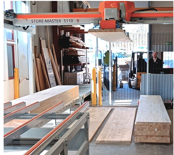
The crane stacks plates into 5 piles made of the same size and material.
