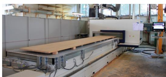
producing several posts simultaneously. Only when the machine has finished all steps with one tool on all posts, the tool is changed and the machine proceeds to the next step with the new tool. The processing of 4 posts now takes about the same amount of time than 2 posts required before Luxholm made the change.
