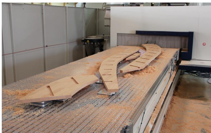
The maximum capacity on the machine is 8 stringers at a time. A possibility that promises future potential timesaving.
