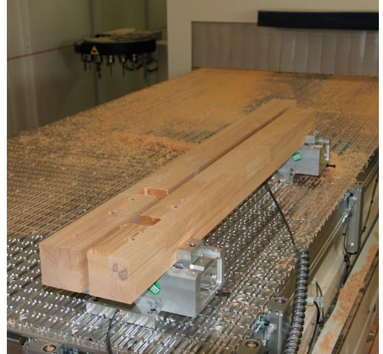
Since the processing of posts generally requires many tool changes, the stair builder saves even more time by utilizing tool optimization and producing several posts simultaneously.
