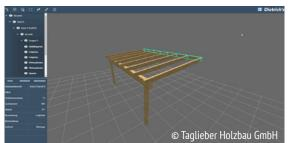
The Compass Software postprocessor automatically transfers all CAD data from the Dietrichs's system to the CNC machine
