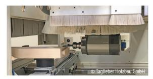
The integrated Compass Software solution enables the woodshop to process different parts on only one machine.
