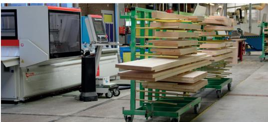
From the moment the order comes in, to its delivery, the production is based on complete orders. All parts of the staircase are kept together as one group.
