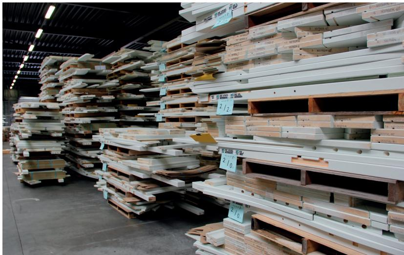
From the moment the order comes in, to its delivery, the production is based on complete orders. All parts of the staircase are kept together as one group.
