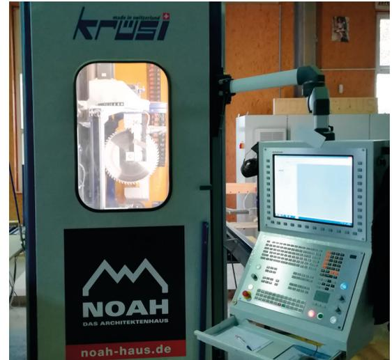
After import of the construction data, the individual parts are prepared for the CNC in a self-determined order, the CNC programs are generated fully automatically, and they are transferred to the machine.
